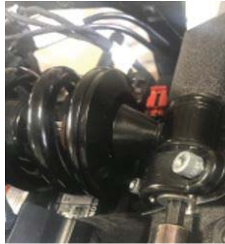
Bushings and shouldered sleeves in rod end of shock assembly (pre installed)
