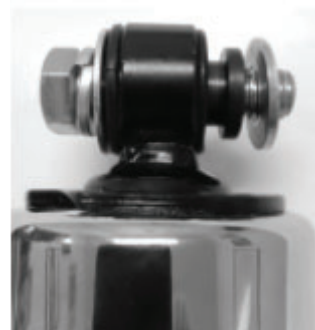
Photo 2 - Install a shouldered sleeve as shown into each mounting eye of both shocks. Also use one 1/2" SAE flat washer in conjunction with the shouldered sleeve to provide sufficient space between the shocks and the Frame / Swing arm.
