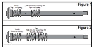
Prior to installing your Slammer Fork Lowering kit, you MUST REMOVE any previously installed fork lowering kit components, such as the 1 or 2 additional top out springs illustrated above. Additional top out springs are common in many such kits.
