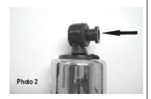
On 1991 - Later Sportsters use an additional spacer in conjunction with the shouldered sleeve to provide sufficient space between the shocks and the frame/swing arm.
