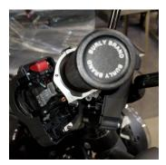
7. Make sure the Flange of the throttle grip fits within the throttle switch housing.
