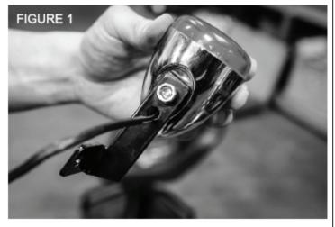
Mount the turn signal to the supplied turn signal bracket using the 5/16-18 x 5/8" bolt (shortest bolt).
