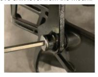
3. Remove shifter ball rod end from the connecting rod.
