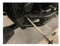
2. Remove clevis pin from master cylinder and the two springs attached to the brake lever. Remove brake lever using external snap ring pliers.
