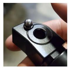
3. Verify the footpeg can move up and down and the detent system is working properly.
