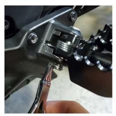
3. Transfer the spring to the Burly foot peg, pay close attention to the orientation of the spring. Place the peg between the clevis, insert the joint pin. Place the thin washer on the end and install the cotter pin, bend the cotter pin to prevent it from backing out.
