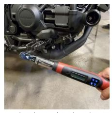
If you need to change the orientation on the pegs be sure to reapply high strength thread locking compound and retorque to 25 ft-lbs
