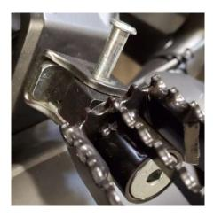
2. Trasnfer the spring, ball and detent plate to the Burly peg. Insert the assembly into the clevis. Insert the joint pin and thin washer then install the cotter pin, bend the cotter pin to prevent it from backing out.
