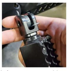
4. Verify the footpeg can move up and down and springs back to its neutral position.
