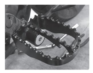
■ Passenger Peg Installation - Reusing the factory compression spring and ball, install spring and ball onto the peg mounting bolt. Using pliers to pinch the ball into peg mounting bolt may allow the peg to go into the clevis peg mount easier.
