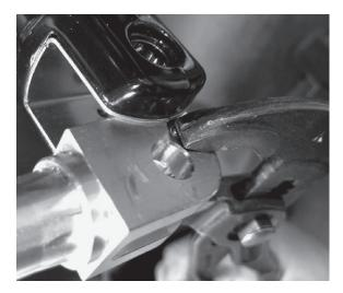
For Models containing an inner sleeve in the clevis peg mount, remove the sleeve from the clevis peg mount before installing the peg mounting bolt. This may ease the installation of the ball and compression spring into the clevis peg mount.
