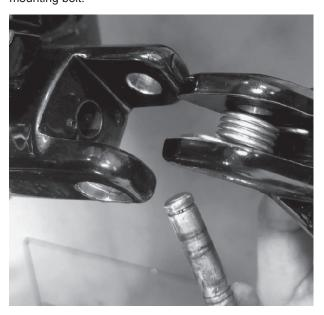
Align peg mounting bolt holes, clevis peg mount and torsion spring. Insert pin and secure with retaining ring.
