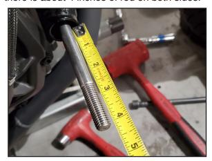
3. Install the new aluminum standoff on both sides of the frame.
