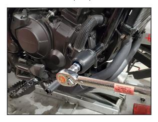
**NOTE:** On the Honda Rebel 1100 DCT version, the plastic engine guard may need to be removed, pushed aside, or modified to install the aluminum standoff. See below.
