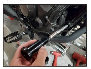
4. Install the Delrin frame sliders and orient the logo to your preference. Refer to the Honda service manual for torque specifications.
