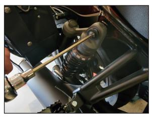
2. Using the supplied bolt and washer, torque to Honda specification. Refer to the Honda service manual for torque specifications.
