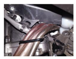
4. Remove the 2 bolts holding the stock cover. The cover and bolts will not be reused, but the steel chain guard will.
