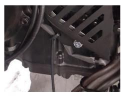
11. Route supplied zip tie around wires and cables routed toward the front of the cover.
